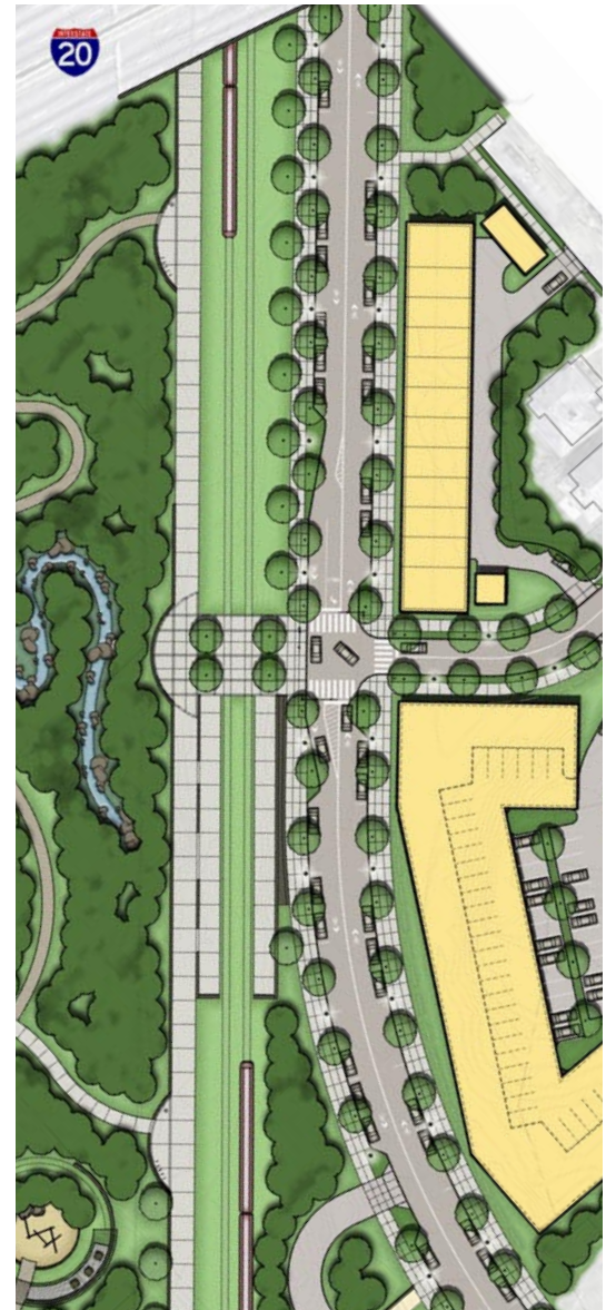
above right: Aerial view of the road diet at Langhorn Street and Lucile Avenue right: Improvements will stretch from I-20 south to R.D. Abernathy Boulevard below: The number of lanes will be reduced from six to two, to accommodate wider sidewalks, tree plantings, parallel parking, and redevelopment
